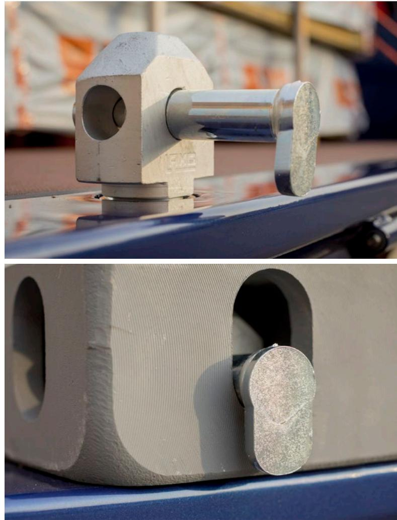
In the case of container freight, all securing of the load is performed from above.
