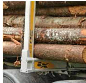
Easy adjustment of the angle between the bolster and stanchions maximises loading capacity when transporting different types of load, for example sawn timber.
