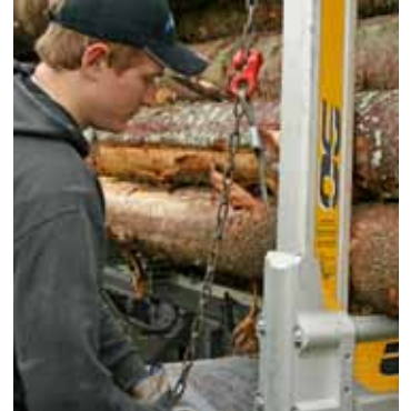
The new auto-tensioner makes the job far easier. The hook is now down on the bolster, and you can lash the load securely without having to stretch and attach the hook high up the chain.
